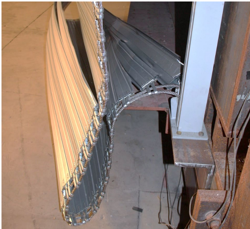
Figure 53. Test 05 - Post-Test Photos of Curtain Shoes
