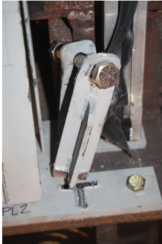
Figure 50. Test 05 - Post-Test Photos of Left Baseplate
