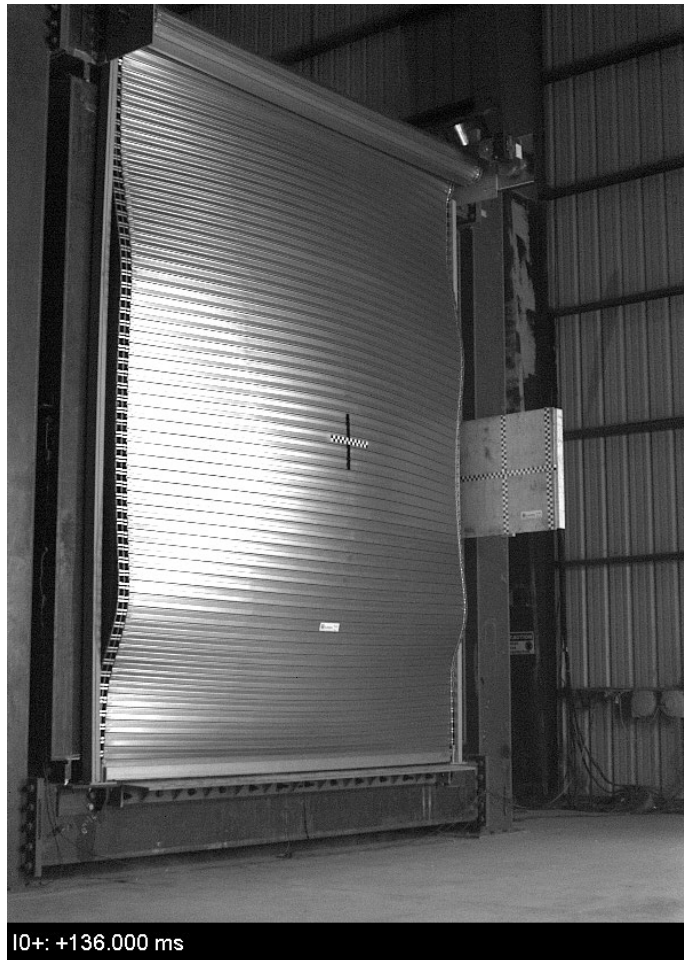
Figure 31. Test 01 - Point of Maximum Deflection (Oblique View)
