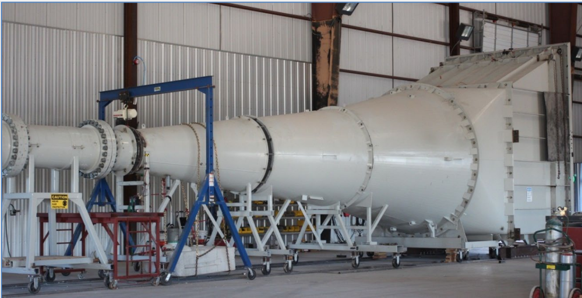
Figure 2. ABS Consulting Shock Tube Apparatus
