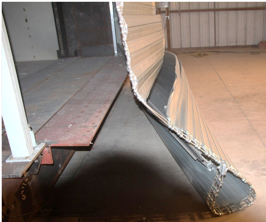
Figure 51. Test 05 - Post-Test Photos of Left Curtain Side
